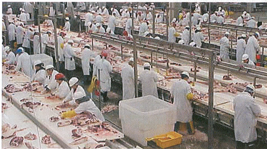
The fabrication tables at Brawley Beef are designed with limited crevices to eliminate pathogen harborage.
