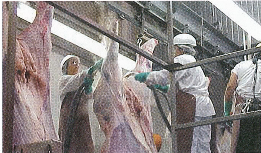
Steam vacuuming is just one of several interventions use by Brawley Beef to keep pathogens at bay in the industry's newest beef-processing facility.
